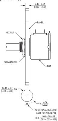
Anti-rotation pin hole is shown at six o'clock position for reference only. The actual location is determined by the customer's application. Refer to the front view of the potentiometer to see the location of the optional A/R pin.
