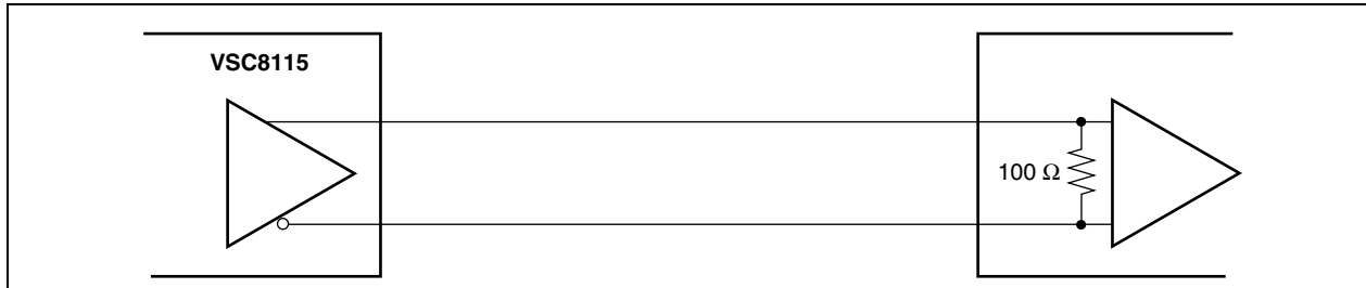
Figure 4. High-Speed Outputs, LVDS Termination
