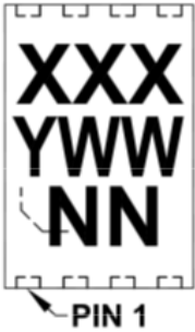
8-Lead DFN (2x3x0.9 mm)
