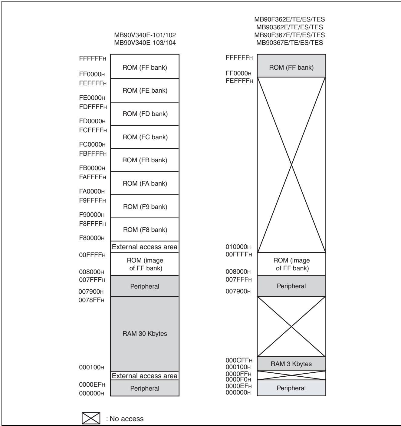
Note: The high-order portion of bank 00 gives the image of the FF bank ROM to make the small model of the C compiler effective. Since the low-order 16 bits are the same, the table in ROM can be referred without using the far specification in the pointer declaration.
