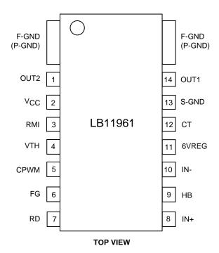
F-GND (P-GND): The motor system ground and the heat sink. Since the heat generated Since the heat generated by the chip is dissipated through F-GND, the thermal resistance is lowered by increasing the area of the copper foil and solder surface in the printed circuit pattern.
