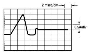
Fig. 6a. Switch-on pulse and steady-state current, example #6
