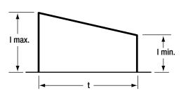
Fig. 3a. Trapezoidal pulse paramerters for Joule integral calculation, example #3
