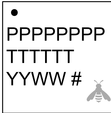
Figure 8.3. QFN24 Package Marking
