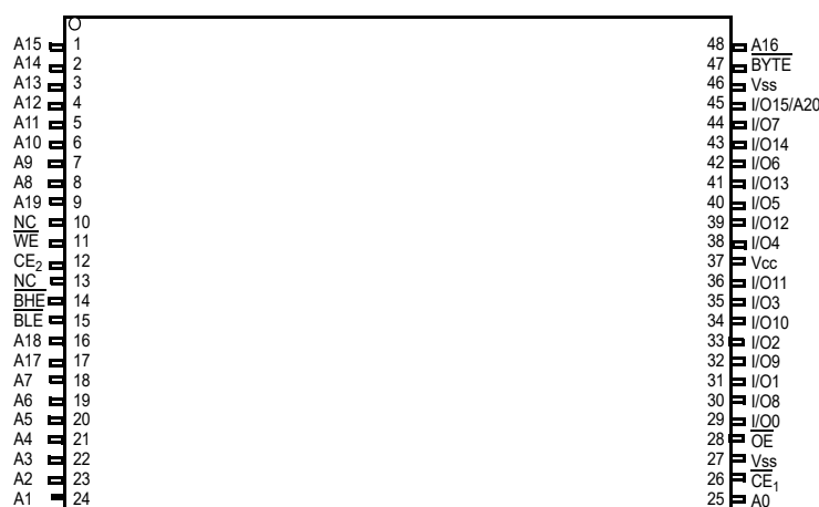
Figure 2. 48-pin TSOP I Pinout (Top View) [2, 3]
