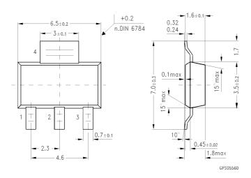
Definition of soldering point with temperature T<sub>s</sub>: upper side of solder edge of device pin 4.
