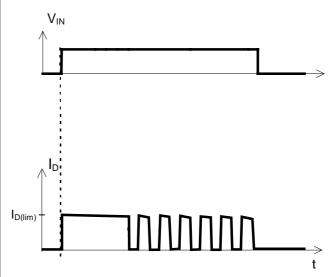
Shut down by overtemperature and restart by cooling. Current internally limited at  $I_{D(lim)}$ .
