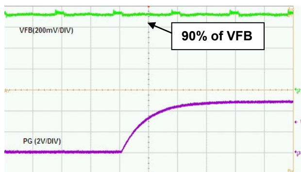
Time- 1µs/div Powergood Rising Threshold
