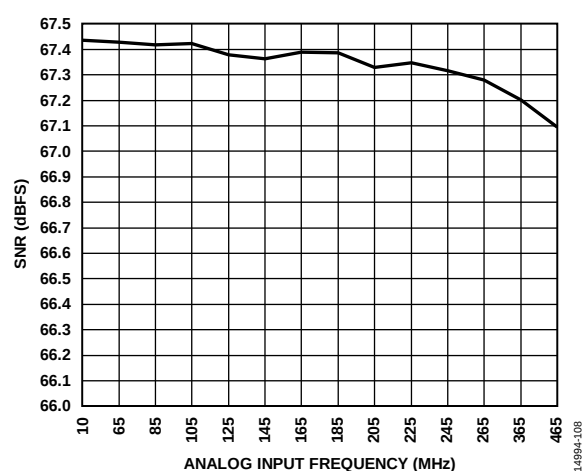
Figure 14. SNR vs. Analog Input Frequency ( f_{IN} ), First and Second Nyquist Zones; A_{IN} at -3 dBFS
