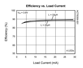
Efficiency vs. Load Current
