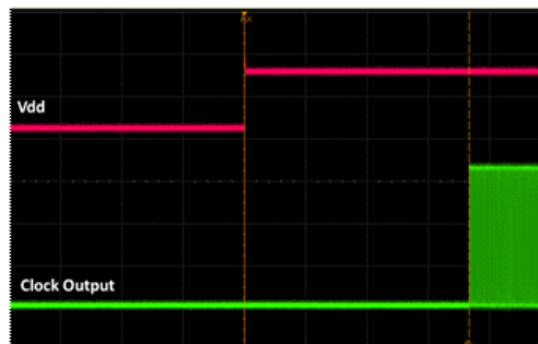
Figure 16. Startup Waveform vs. Vdd
