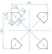
The positive polarity terminal: 1 The negative polarity terminal: 2=3=4 common Dimensions in mm
