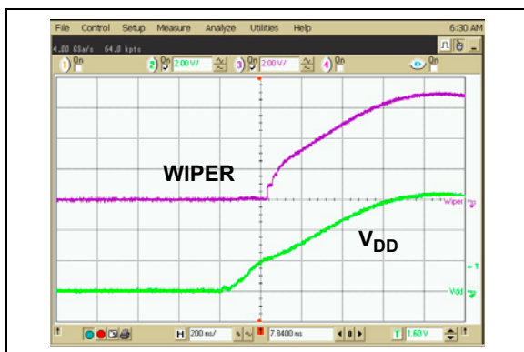
FIGURE 2-15: 2.1 k \Omega – Power-Up Wiper Response Time.
