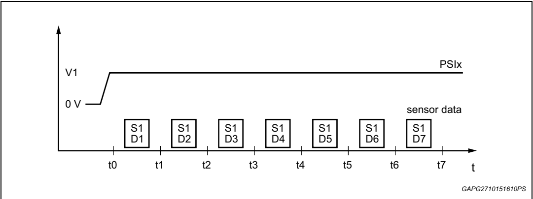
Figure 17. Sensor buffer in asynchronous mode diagram
