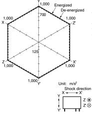
Test Item: G5NB-1A-E, 24VDC Number of Relays: 5 pcs Test Method: Shock was applied 3 times in 6 directions along 3 axes and the level at which shock caused malfunction was measured. Rating: 100 m/s<sup>2</sup>
