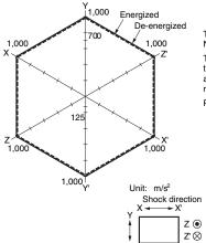
Test Item: G5NB-1A, 24VDC Number of Relays: 5 pcs Test Method: Shock was applied 3 times in 6 directions along 3 axes and the level at which shock caused malfunction was measured. Rating: 100 m/s<sup>2</sup>
