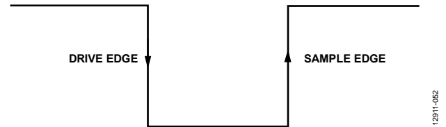
Figure 42. SPI Mode 3 SCLK Edges
