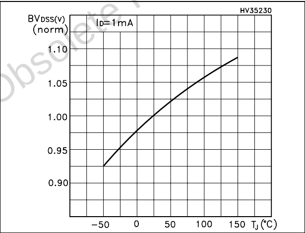
Figure 17. Normalized BV_{DSS} vs temperature
