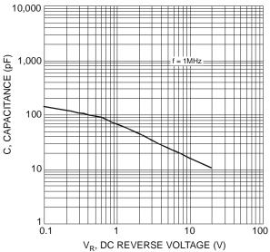
Fig. 4 Total Capacitance vs. Reverse Voltage
