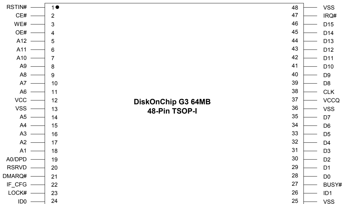
Figure 1: TSOP-I Pinout for Standard Interface (DiskOnChip G3 64MB/512Mb)
