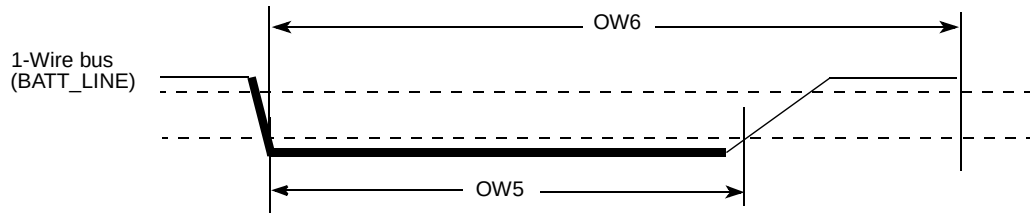
Figure 7. Write 0 Sequence Timing Diagram
