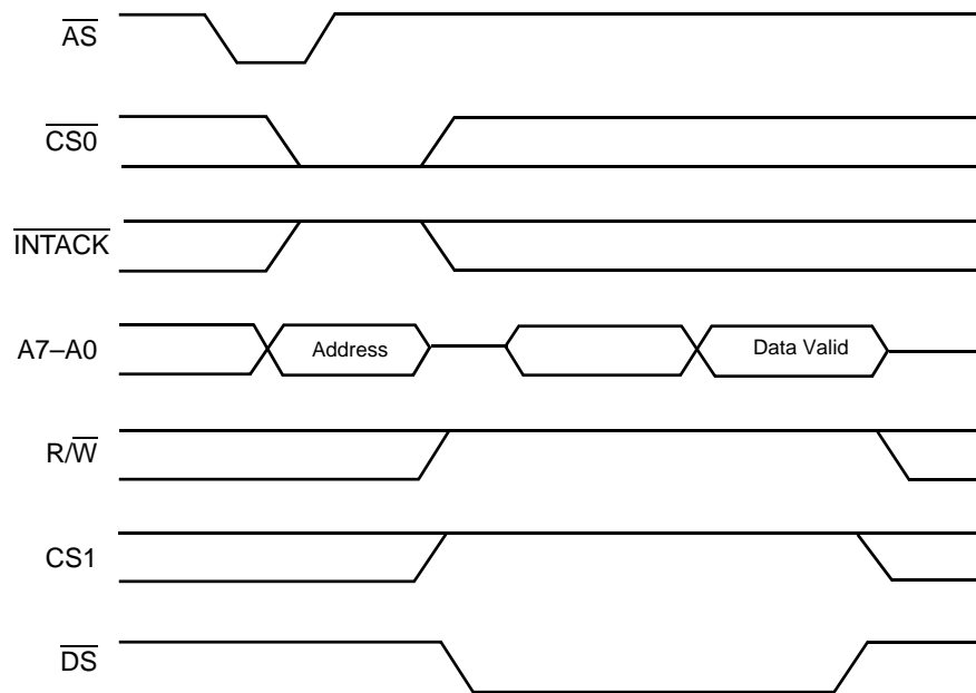
Figure 18. Z80230 Read Cycle Timing
