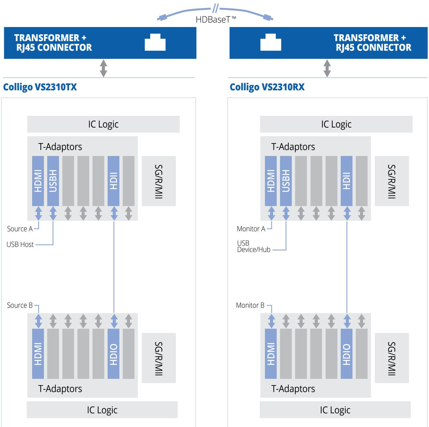
The following diagram illustrates the HDBaseT™ Gen 2.0 in a signage daisy chain system:
