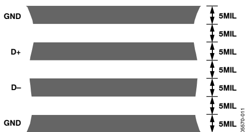
Figure 22. Typical Arrangement of Signal Tracks
