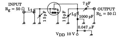
$L_1$ : 1.0 mm $_{\phi}$  silver plated copper wire 4.0 T, 8 mm $_{\phi}$  ID TAP at 1.0 T from coil end
