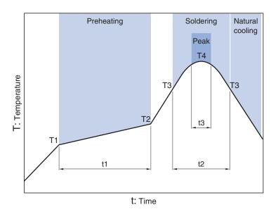
Preheating Soldering Peak Time Temp. Time Temp. Temp. Time Τ1 T2 t1 тз t2 Т4 t3 150°C 180°C 60 to 120s 230°C 30s 260°C 10s
