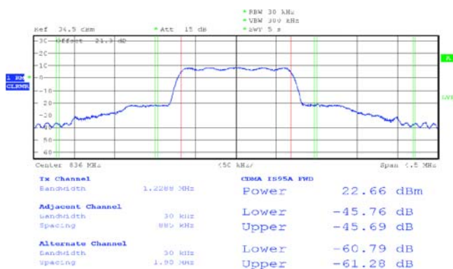
ACPR, IS-95 FWD, V_{CC} 3.5 V, V_{APC1, 2} = 2.7 V 836 MHz @ 25 °C
