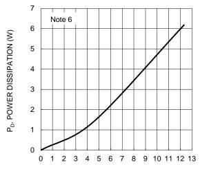
$I_{F(AV)}$ , AVERAGE FORWARD CURRENT (A) Figure 1. Forward Power Dissipation
