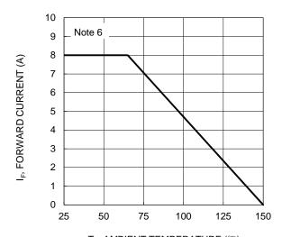
$\mathrm{T_{A}},\,\mathrm{AMBIENT}\,\mathrm{TEMPERATURE}\;(^{\circlearrowright})$  Figure 4. Forward Current Derating Curve
