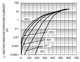
V<sub>F</sub>, INSTANTANEOUS FORWARD VOLTAGE (mV) Figure 2. Typical Forward Characteristics
