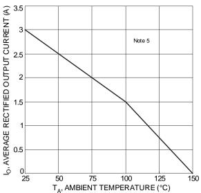
Figure 5 Forward Current Derating Curve
