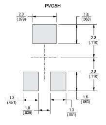
DIMENSIONS:  $\frac{\text{MM}}{(\text{INCHES})}$  TOLERANCES:  $\pm \frac{0.1}{(.004)}$  EXCEPT WHERE NOTED
