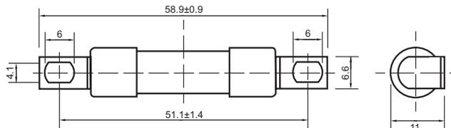
**Cylindrical with PCB tabs PV-(amp)A10-1P (single pin), PV-(amp)A10-2P (double pin)**
