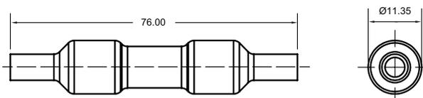
The in-line crimp terminal version can be electrically insulated with customer supplied overmolding or approved heat-shrink.
