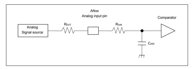
(Equation 1) t<sub>S</sub> ≥ (R<sub>AIN</sub> + R<sub>EXT</sub>) × C<sub>AIN</sub> × 9
