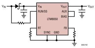
Figure 2. The Input Diode Prevents a Shorted Input from Discharging a Backup Battery Tied to the Output. It Also Protects the Circuit from a Reversed Input. The LTM8050 Runs Only When the Input is Present
