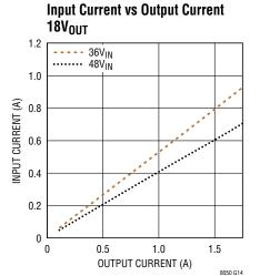
Output Current vs V<sub>IN</sub> Output
