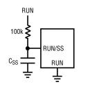
Figure 1. Apply an RC Network to RUN/SS to Control the Soft-Start Behavior of the LTM8050 at Power-Up
