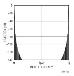
Figure 26. Sinc<sup>4</sup> Filter Rejection
