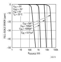
Figure 19. Full-Scale Error vs R<sub>SOURCE</sub> (Small C)
