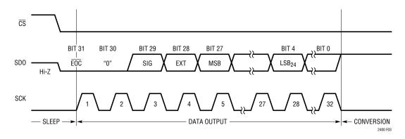
Figure 3. Output Data Timing
