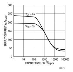
Figure 14. CS Capacitance vs Supply Current
