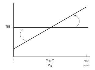
Figure 16. Offset/Full-Scale Shift
