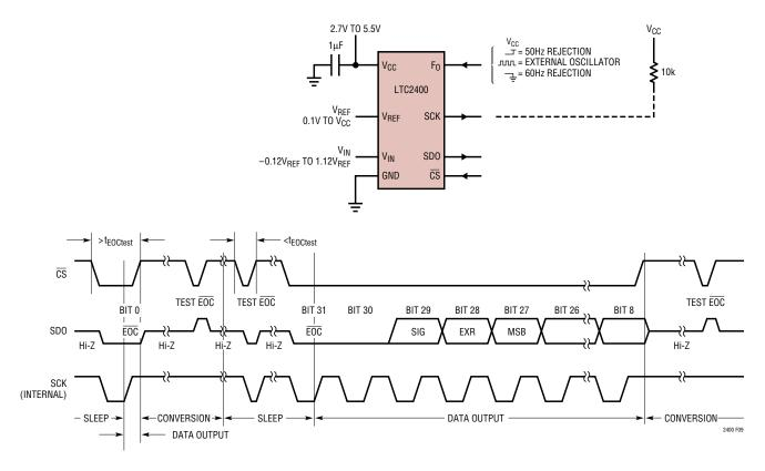
Figure 9. Internal Serial Clock, Reduced Data Output Length
