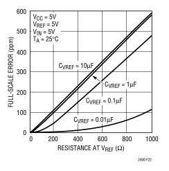
Figure 22. Full-Scale Error vs R<sub>VREF</sub> (Large C)
