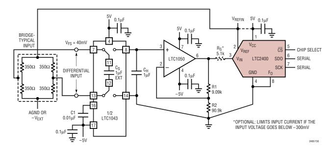
Figure 30. Differential to Single-Ended Converter for Low Level Inputs, Such as Bridges, Maintains the LTC2400's High Accuracy
