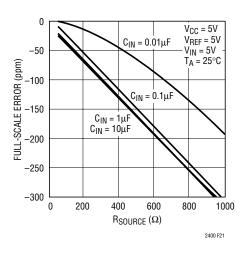
Figure 21. Full-Scale Error vs R<sub>SOURCE</sub> (Large C)
