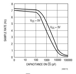
Figure 13. CS Capacitance vs Output Rate
