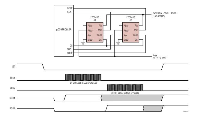
Figure 27. Synchronous Conversion—Extendable
