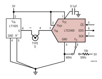
Figure 37. The LT1025 Complete Cold Junction Solution
