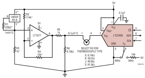
\*RECOMMENDED 0.1%, ±5ppm IRC AFD SERIES CHIP RESISTORS
