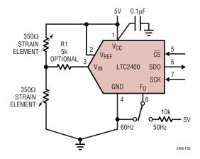
Figure 40. Half-Bridge Connection for Strain Gauges
