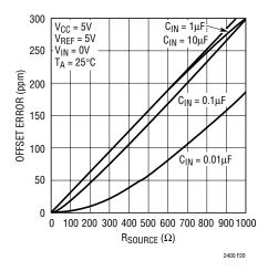
Figure 20. Offset vs R<sub>SOURCE</sub> (Large C)
