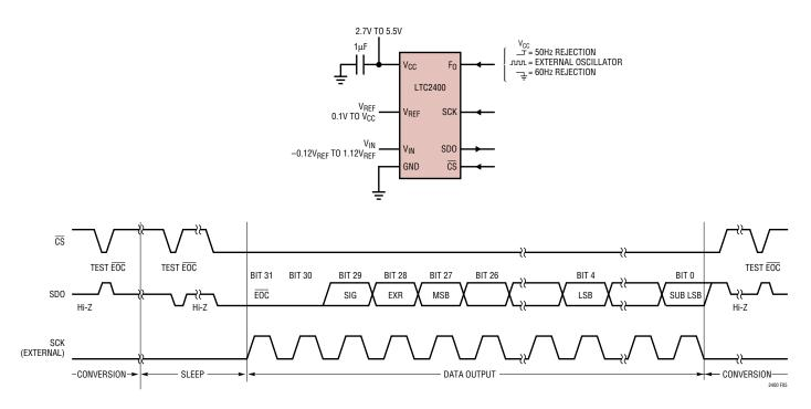
Figure 5. External Serial Clock, Single Cycle Operation
