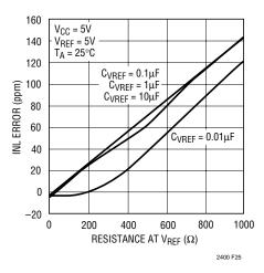
Figure 25. INL Error vs R<sub>VREF</sub> (Large C)
