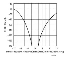
Figure 4. LTC2400 Normal Mode Rejection When Using an External Oscillator of Frequency f<sub>EOSC</sub>
