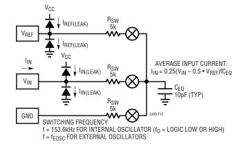
Figure 15. LTC2400 Equivalent Analog Input Circuit
