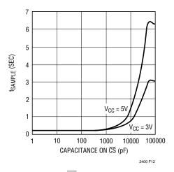
Figure 12. CS Capacitance vs t<sub>SAMPLE</sub>
