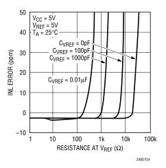
Figure 24. INL Error vs R<sub>VRFF</sub> (Small C)
