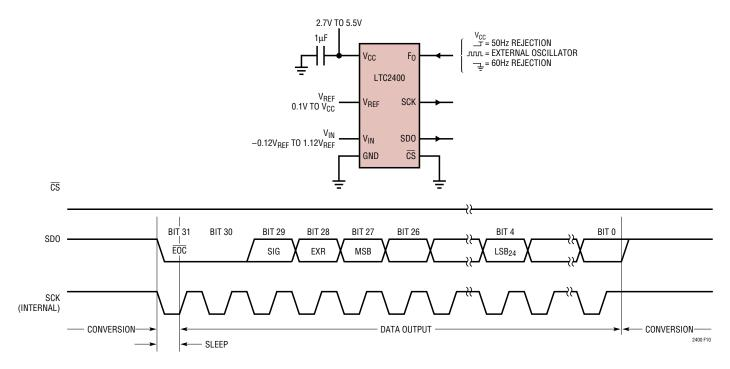
Figure 10. Internal Serial Clock, Continuous Operation
