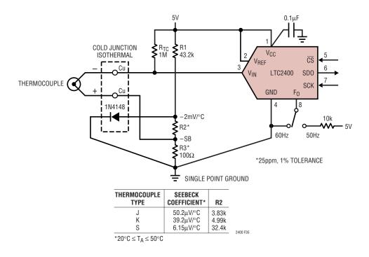
Figure 35. Diode Cold Junction Compensation
