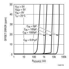
Figure 18. Offset vs R<sub>SOURCE</sub> (Small C)
