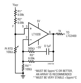
Figure 39. Extremely High Resolution RTD Interface
