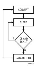
Figure 1. LTC2400 State Transition Diagram
