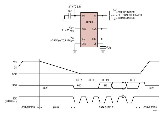
Figure 11. Internal Serial Clock, Autostart Operation
