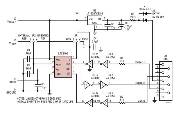
Figure 42. 24-Bit A/D Demo Board Schematic
