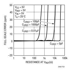
Figure 23. Full-Scale Error vs R<sub>VRFF</sub> (Small C)
