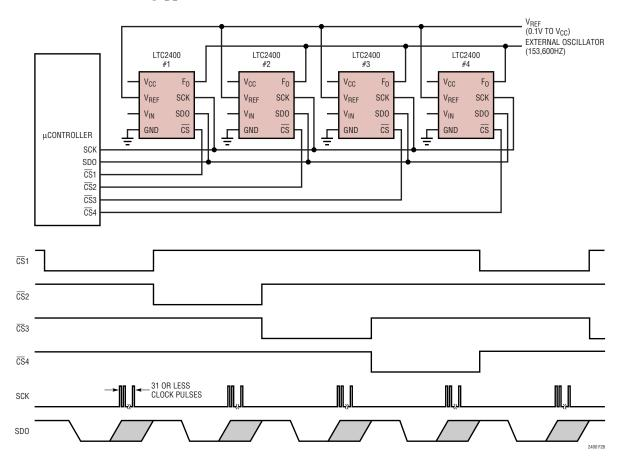
Figure 28.  $4 \times$  Output Rate LTC2400 System
