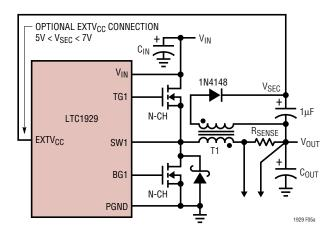
Figure 5a. Secondary Output Loop with EXTV<sub>CC</sub> Connection
