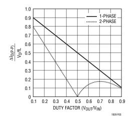
Figure 3. Normalized Output Ripple Current vs Duty Factor  $[I_{RMS}\approx 0.3~(\triangle I_{0(P-P)})]$
