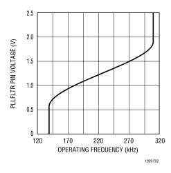
Figure 2. Operating Frequency vs V<sub>PLLFLTR</sub>
