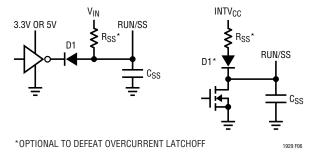
Figure 6. RUN/SS Pin Interfacing
