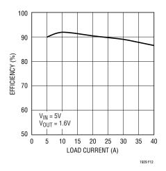
Figure 12. Efficiency Plot for Circuit of Figure 11
