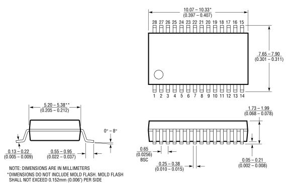
\*\*DIMENSIONS DO NOT INCLUDE INTERLEAD FLASH. INTERLEAD FLASH SHALL NOT EXCEED 0.254mm (0.010") PER SIDE
