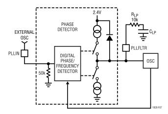
Figure 7. Phase-Locked Loop Block Diagram
