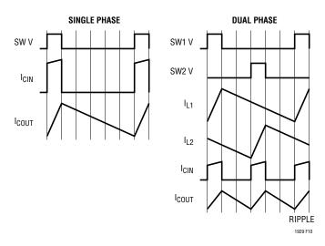
Figure 10. Single and 2-Phase Current Waveforms
