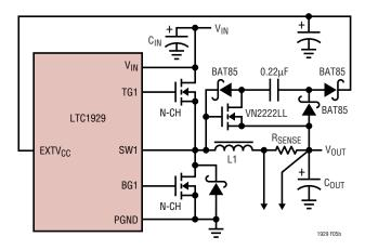
Figure 5b. Capacitive Charge Pump for EXTV<sub>CC</sub>
