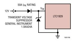
Figure 8. Automotive Application Protection
