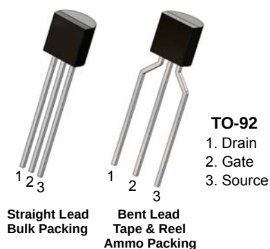
Figure 1. J175 / J176 Device Package
