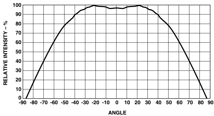
Figure 7. Relative intensity vs. angle for HSMx-C177 and C197.
