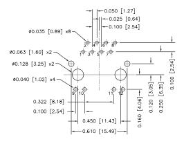
Recommended PCB Layout (Component Side)
