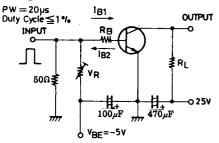
$$\begin{split} I_C \!=\! 10I_{B1} \!=\! -10I_{B2} \!=\! 500\text{mA}, & V_{CC} \!=\! 25V \\ \text{For PNP, the polarity is reversed.} \end{split}$$
