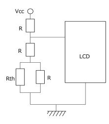
Temperature Compensation (RF circuit)
