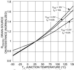
Figure 6 On-Resistance Variation with Temperature
