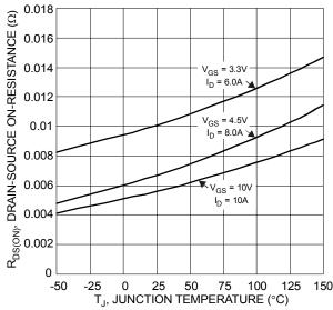
Figure 7 On-Resistance Variation with Temperature
