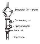
Note: 1. The spring washer comes with the lock nut.
