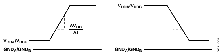
Figure 14. Transient Immunity Waveforms—Output Supplies
