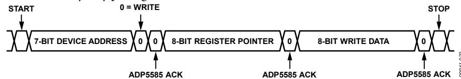
Figure 23. I 2 C Single Byte Write Sequence
