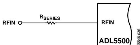
Figure 36. Attenuating the Input Signal
