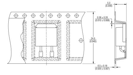
DIMENSIONS:  $\frac{\text{MIM}}{(\text{INCHES})}$ TOLERANCE:  $\frac{\pm 0.38}{(\pm 0.015)}$  UNLESS OTHERWISE NOTED
