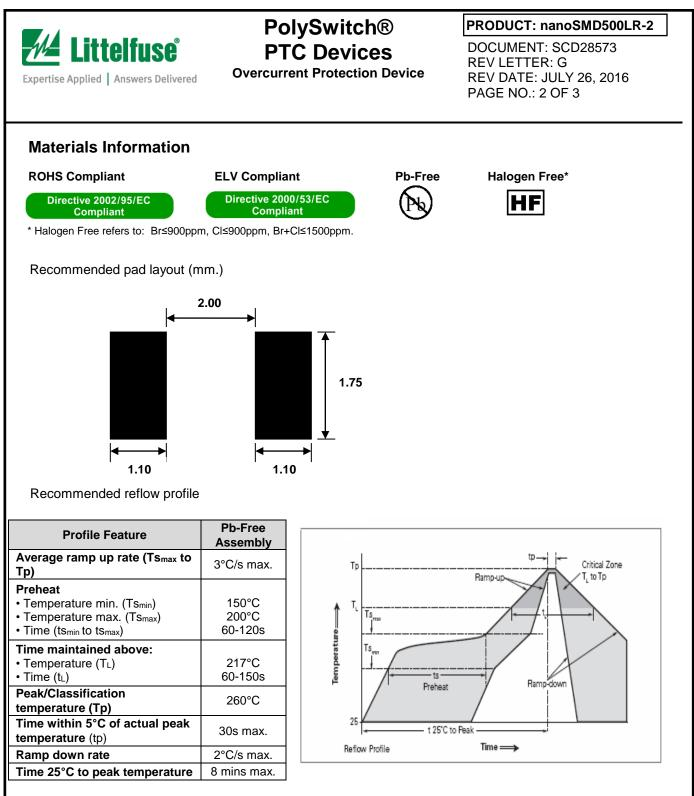
Note: All temperatures refer to top side of the package, measured on the package body surface.
