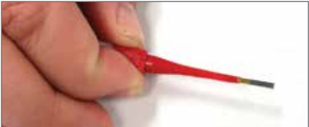
Plastic tool with contact in proper position.
