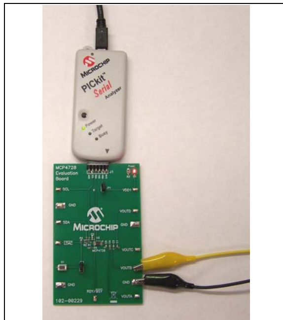
FIGURE 8-2: Setup for the MCP4728 Evaluation Board with PICKit™ Serial Analyzer.
